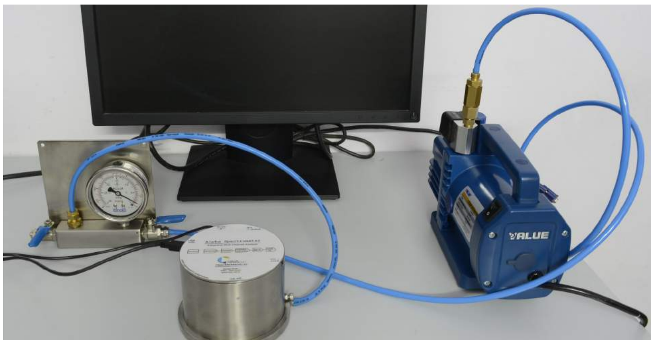
Figure 5: Photo of vacuum pump and pumping assembly connected to the spectrometer
